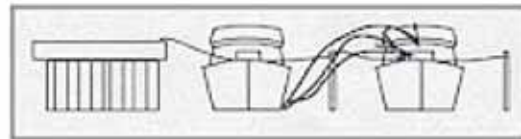
NEARBY BOAT GENERATOR EXHAUST
