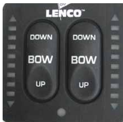
Trim Tab Switches
